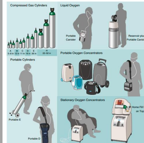
Figure 1. Examples of stationary and portable oxygen devices in the United States. Illustration by Patricia Ferrer Beals.
