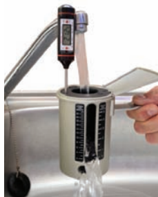
A flow cup gives litres per minute readings
