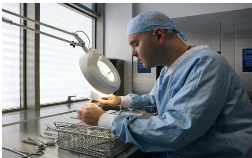
Figure 16.1: Post cleaning inspection
