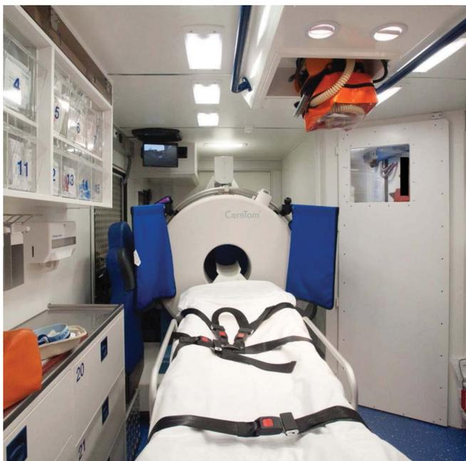
Note the CT scanner in the back of the cabin and the separated shielded workstation on the right behind the door.
